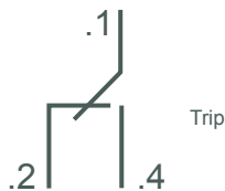
Terminal Designations and Function of General Purpose Alarm Switch
